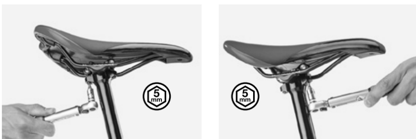
Figure 6. Tightening / loosen single saddle bolt
