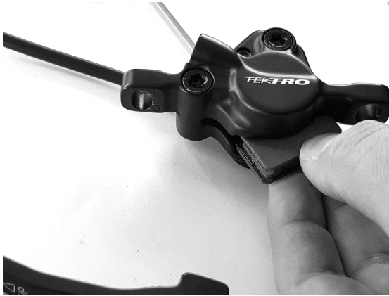
Figure 23: Gently push at the top of the pads and the pads should slide out
