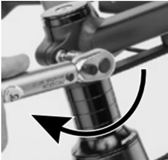
Figure 10. Retighten the stem bolts to 5nm
