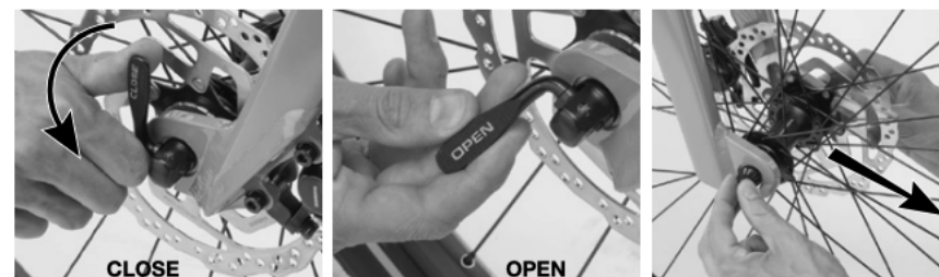
Figure 14: Stages of tightening the axle.
