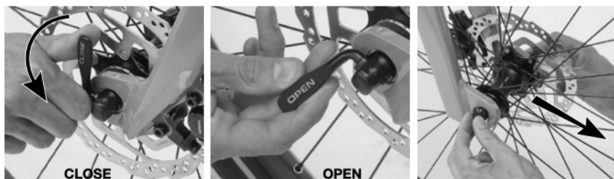
Figure 13. Stages of opening the quick release axle
