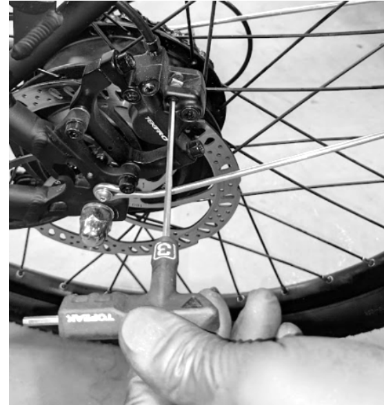
Figure 22: Undo pad retaining bolt
