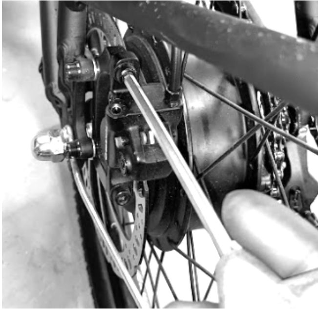
Figure 21: Undo the mount bolts to remove calliper
