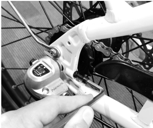
Figure 16: Set axle tension by turning bolt clockwise. Ensure the bolt on the opposite side is also set.
