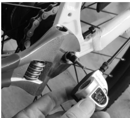
Figure 19: Adjustment of axle nut drive side
