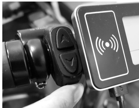
Figure 36: Press and hold to turn off again
