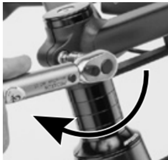
Figure 10. Retighten the stem bolts to 5nm
