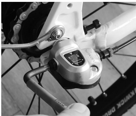
Figure 18: Turn the m5 shifter nut anti-clockwise. After a few rotations the mechanism pulls off
