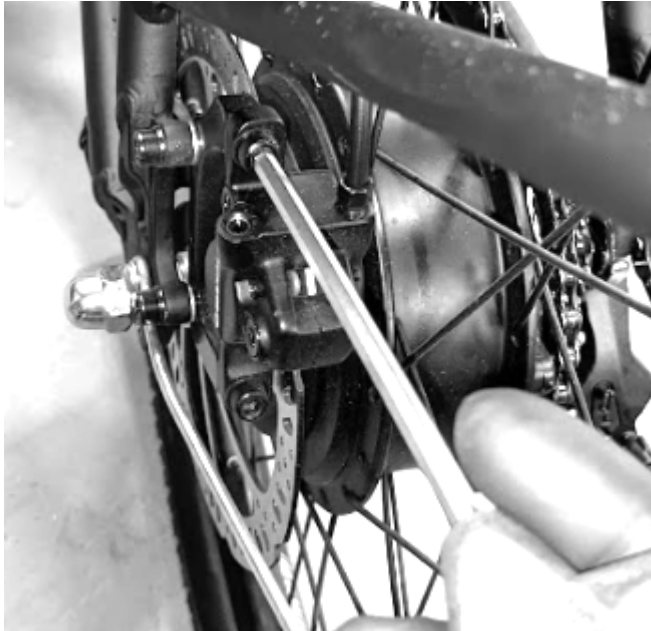
Figure 27: Undo the mount bolts to remove calliper
