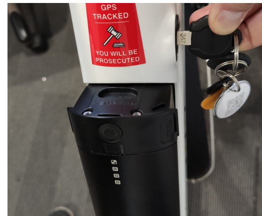
Figure 38: Removing the battery
