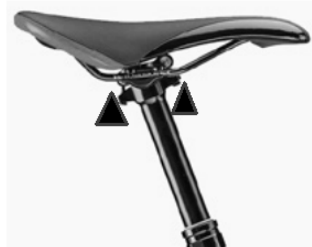
Figure 4. Intermediate saddle setback position
