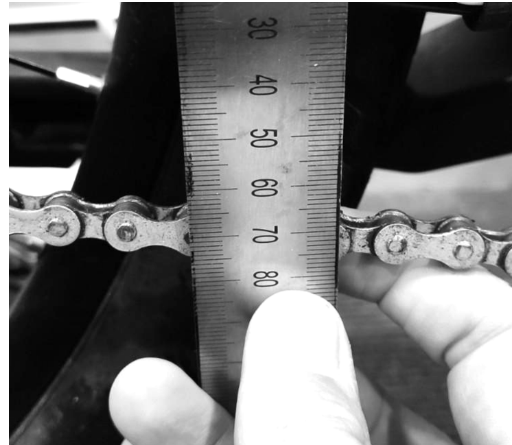
Figure 22: The chain should not have more than 1cm of flex either side of the resting position of the chain. If it can be pushed further the chain will need to be tightened.
