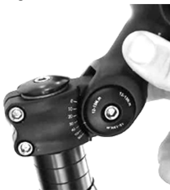
Figure 12. Adjusting the stem to position
