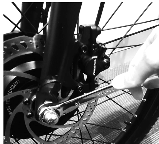
Figure 15: Tighten nut to 35nm
