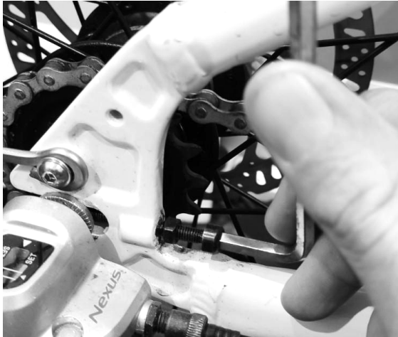
Figure 23: Turn the hex bolt clockwise which will add tension to the chain
