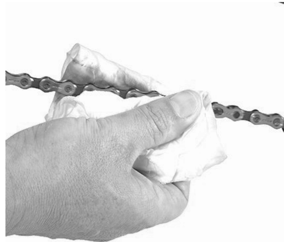
Figure 25: Use a cloth to remove debris and dirt from the chain. Gently turn the pedal with the rear wheel elevated for cleaning. Soapy water is the best cleaning solution. Avoid heavy degreasers where possible.
