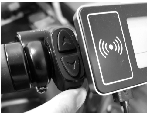
Figure 32: Press the display on button until screen lights up
