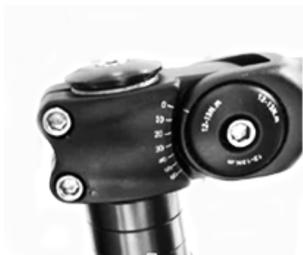
Figure 11. Loosen the M5 Bolt (center)
