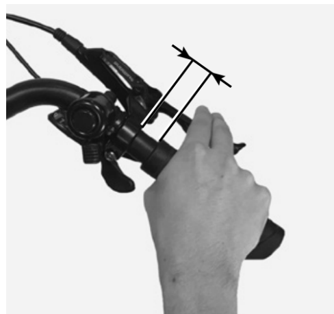
Figure 8. Distance between lever and grip
