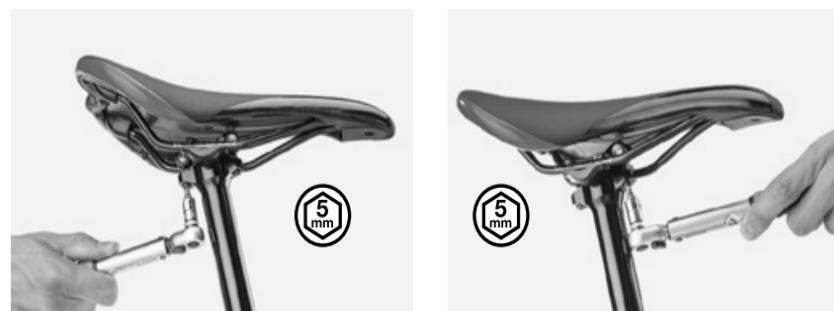
Figure 6. Tightening / loosen single saddle bolt
