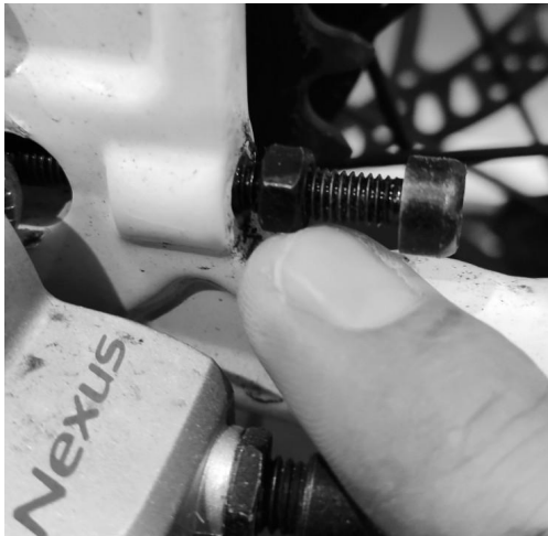
Figure 24: Ensure the retaining nut is tightened against the frame to stop axle movement.
