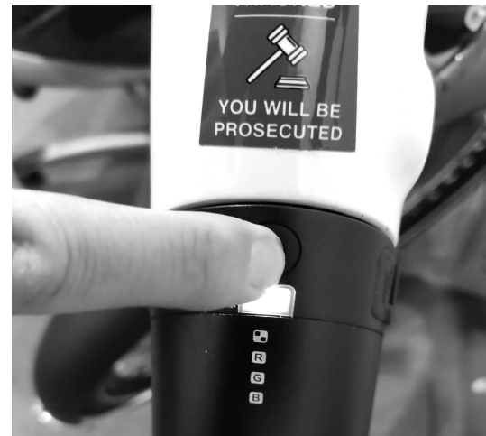
Figure 31: Press and hold button to turn on
