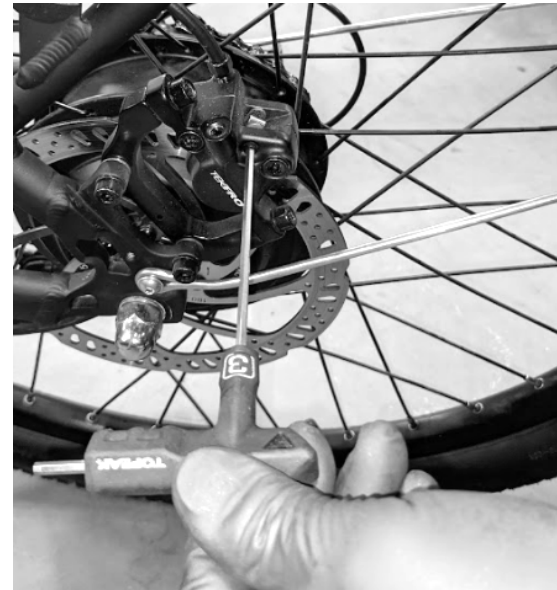
Figure 28: Undo pad retaining bolt
