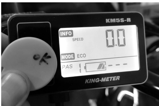
Figure 33: Scan the yellow RFID to enable system
