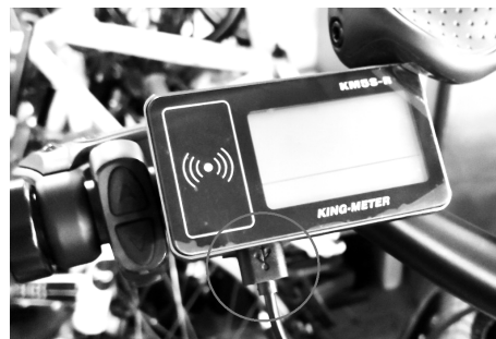
Figure 34: The USB device plug is under the screen
