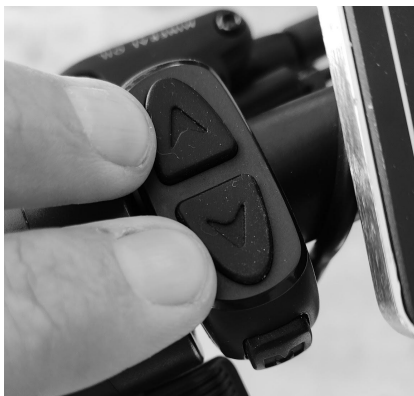
Figure 35: The control pad pedal assist up / down
