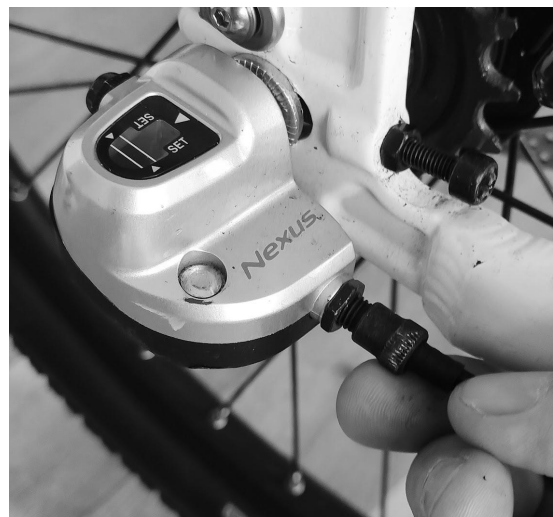
Figure 21: Adjust the barrel by turning either way
