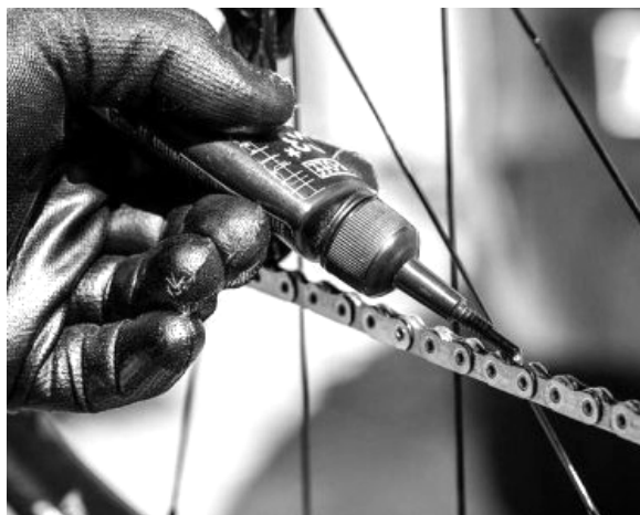
Figure 26: Apply 3-4 drops of dry lubricant to the chain
